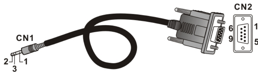
Figure C-2: Adapter Cable for COM1 - Connector Pinouts
